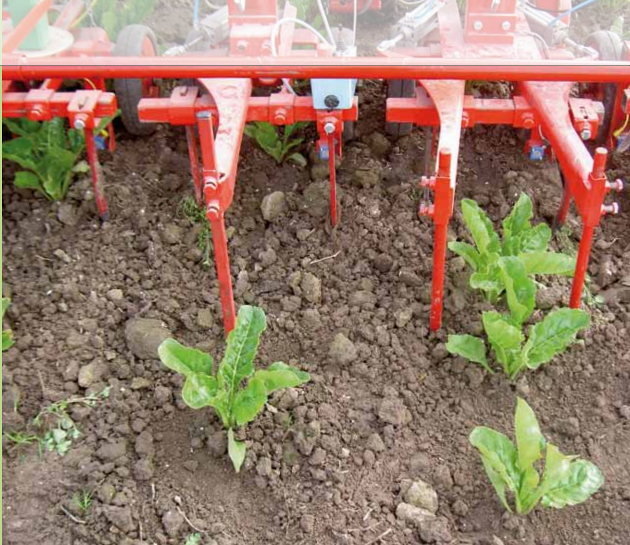
Intra-row weeding with one hoe per row on the left and two hoes per row on the right
