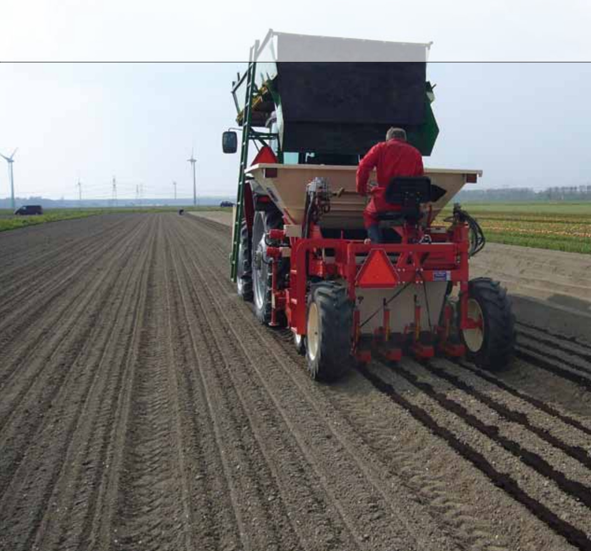
Machine which simultaneously sows and deposits a compost layer to prevent the emergence of weeds
